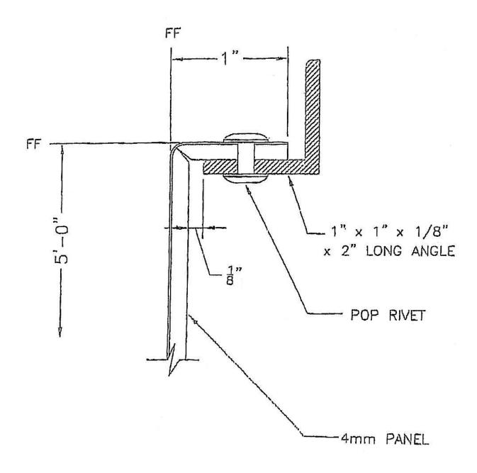
FIGURE 5—ROUT AND RETURN CLIP ATTACHMENT
