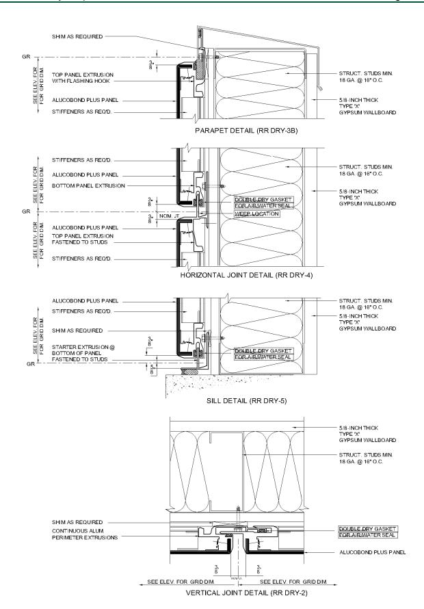
FIGURE 4—DETAILS FOR NONCOMBUSTIBLE ALTERNATIVES - ROUT AND RETURN WITH PERIMETER EXTRUSIONS
