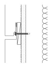
Fig. 1  $\cdot$  Panel Fasteners must fully engage wall framing
