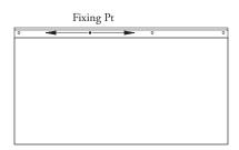
Fig.  $2\cdot$  Each panel should have a single fixing point. The remainder of the holes should be slightly larger than the fasteners.
