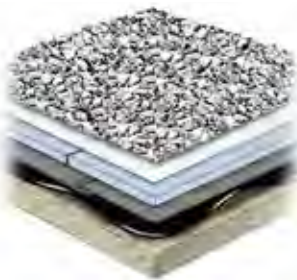
Stone Ballasted Protected Membrane Roof
