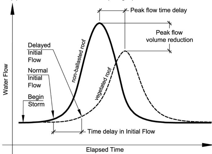
Civil engineers use hydrographs to predict the performance of stormwater BMPs. Comparing hydrographs from non-vegetated and vegetated roofs can determine the delay in the peak flow and the reduction of the peak volume.
