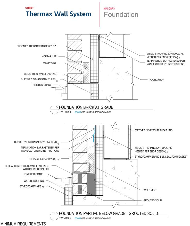
1. OPTIONAL - MIN. 3" WIDTH OF LIGHT GAUGE METAL STRAPPING, MIN. 16" ABOVE GRADE, TO ACT AS NAILING BASE FOR TERMINATION BAR.
