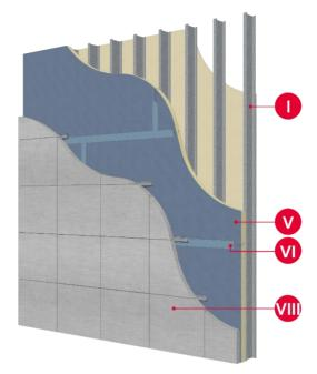
Figure 1 – Typical Layer Assembly
