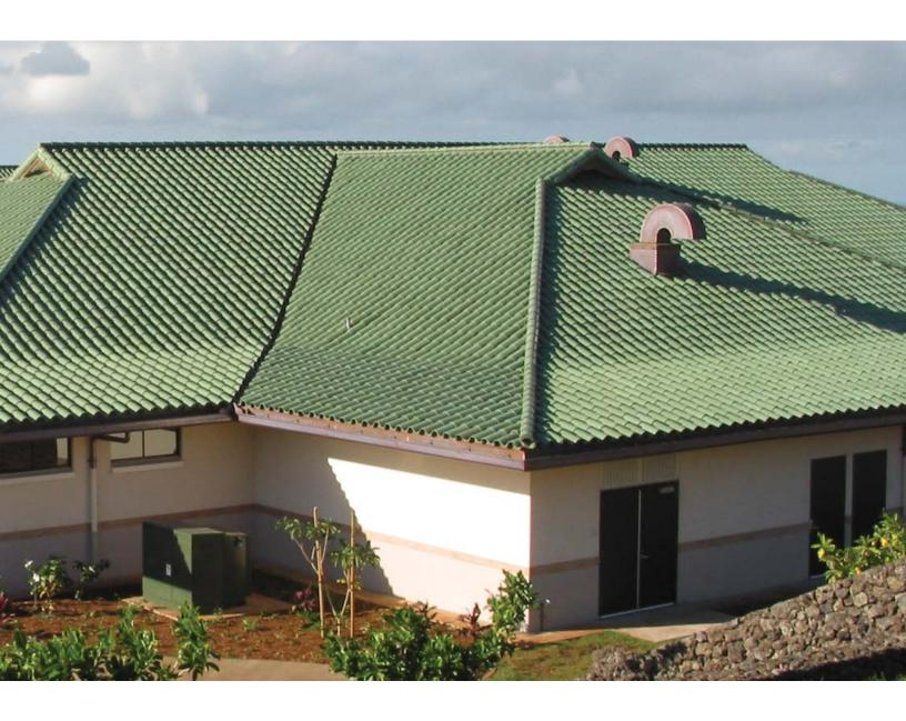
Terra cotta products are naturally green, free from synthetic and toxic materials and can provide energy savings benefits. Rejected or broken terra cotta pieces can be crushed and re-used. At the end of their usable life, terra cotta tiles can be used as drainage fill or landscaping through the existing brick recycling stream.
