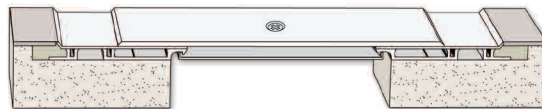
Series LASB / 8" - 24" LASB-Aluminum / LSSB-Stainless / LBSB-Bras / Floor-to-Floor / Seismic Recess Mount Nominal Joint Openings 8" to 24" NOTE: Also available as Floor-to-Wall system
