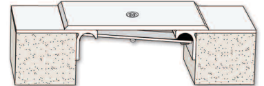
Series ASJ Floor-to-Floor (3" minimum opening) Nominal Joint Openings 3.0" to 18.0" NOTE: Also available as Floor-to-Wall system
