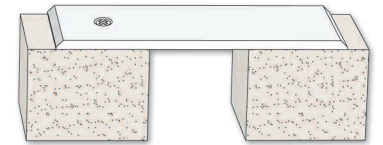
Series SP Floor-to-Floor Nominal Joint Openings 1" to 18" NOTE: Also available as Floor-to-Wall system
