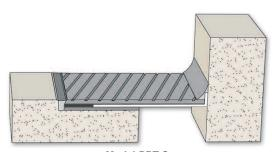
Model PPT-C Slab-to-Wall / Movement .625" to 4.25"
