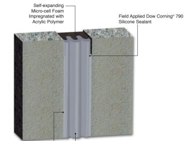
Factory applied Pressure-sensitive sidewall adhesive
